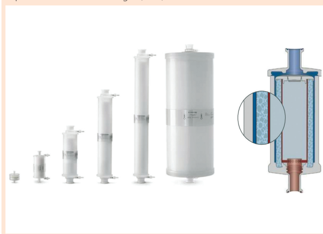
Figure 2: Overview of membrane chromatography capsule portfolio with bed volumes ranging from 3 mL to 5 L and from 1 mL to 2.5 L, with 4-mm and 8-mm bed heights, respectively (LEFT); cutaway view of a 150-mL capsule with 8-mm bed height (RIGHT) with blue and red flow channels
