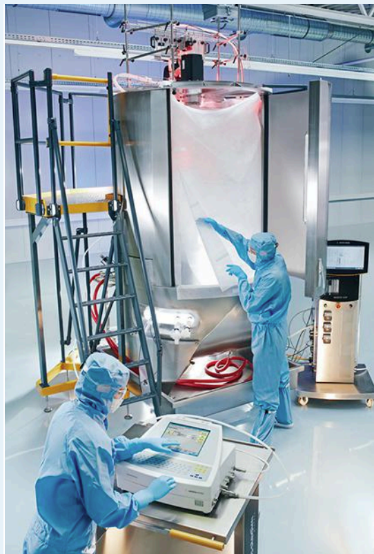
Photo 3: Sartochek 4 Plus bag tester experimental set-up with the BIOSTAT STR 2000
