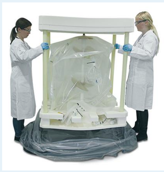
Photo 2: A protective packaging frame prevents contact of sharp objects with the bag film and tubing during transport. Special compartments at the bottom and top separate tubing and connectors from the bag chamber.
