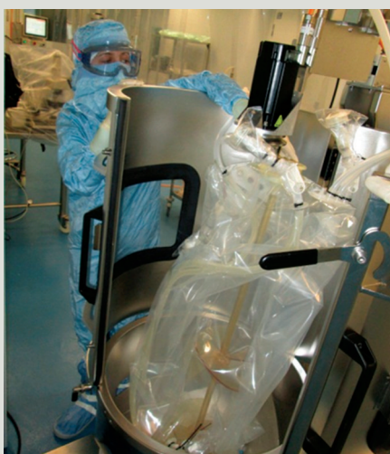
Photos 3 and 4: Installation of a single-use bag in a BIOSTAT STR 200L bag holder (Sartorius Stedim Biotech GmbH)
