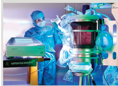
Photo 5: Sartochek 4Plus bag tester connected to CultiBag STR 50L single-use bag (Sartorius Stedim Biotech GmbH)
