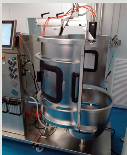
Photos 3 and 4: Installation of a single-use bag in a BIOSTAT STR 200L bag holder (Sartorius Stedim Biotech GmbH)
