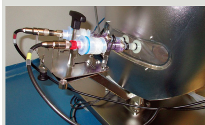
Photo 2: Conventional pH and DO sensors inserted in BIOSTAT STR single-use bioreactor (Sartorius Stedim Biotech GmbH)
