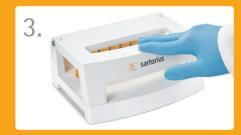
Press down on the station lid so that the left and right corners touch the base plate. Hold the lid in place for 3 seconds to ensure all sample liquid is filtered through.
