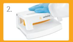
Apply slight uniform pressure with your hand to start sample clarification. You will feel a certain resistance while liquid is pressed through each membrane.
