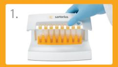
Close the station lid. The grooves align the caps automatically, securely sealing every single Claristep® Filter unit for the most convenient processing.
