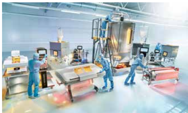
▲ Figure 1. Single-use equipment can include presterilized, disposable bags, tubing, fittings, and connectors. Bioreactor volumes up to 2,000 L are also available for completely single-use cell culture processes.
